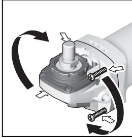
The machine head can be rotated with respect to the machine housing in 90° steps. In this manner, the On/Off switch can be brought into a more convenient position for special working situations, e. g., for cutting operations using the cutting guide with dust extraction protection guard **19** or for left-handed persons.
