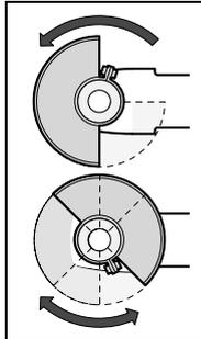
Place the protection guard **7** on the spindle collar. Adapt the position of the protection guard **7** to the requirements of the work step. Lock protection guard **7** by tightening locking screw **20** with combination spanner **4**.
