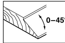
When beveling rebates and surfaces, adjust the required slope angle with the angle adjustment **27**.
