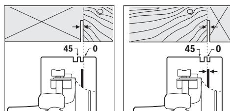
The 0° cut mark (10) indicates the position of the saw blade when making a right-angled cut. The 45° cut mark (9) indicates the position of the saw blade when making a 45° cut. For a precise cut, place the circular saw against the workpiece as shown in the figure. We recommend making a test cut.
